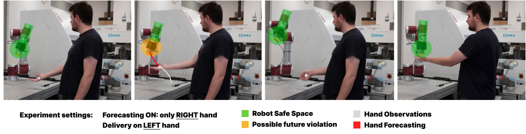
Fig. 5. Example of the framework in a real-world implementation. In this example, the right hand is the only one tracked with the forecasting method. Note that this is a testing choice, not a limitation of the framework. The operator stands in front of the robot, and the hand is tracked in 3D using a Leap Motion V2 device. The device streams the data in real-time to the neural network that predicts the future position of the hand with a 1000 ms time horizon. When the operator moves the robot control, seeing that the hand will collide within the future time horizon, adjusts the planning by keeping a safe distance from the operator's hand. Finally, the delivery is performed on the left hand.
