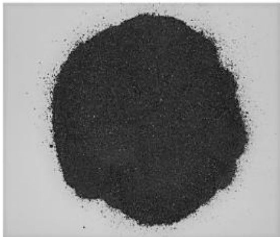
Figure 1. Industrial slag waste after ball milling and sieving.
