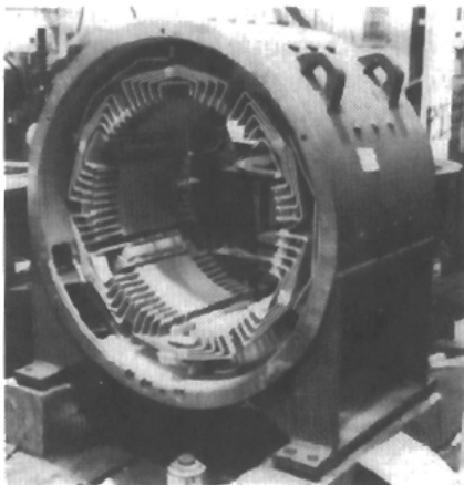
FIGURE 4.33 Compensating winding. (a) Developed diagram. (b) Schematic diagram. (c) Photograph. (Courtesy of General Electric Canada Inc.)
