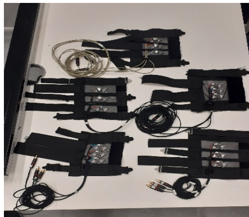
Figure 3. The five vibrotactile sleeves with different interspacings between actuators that were used in the experiment.
