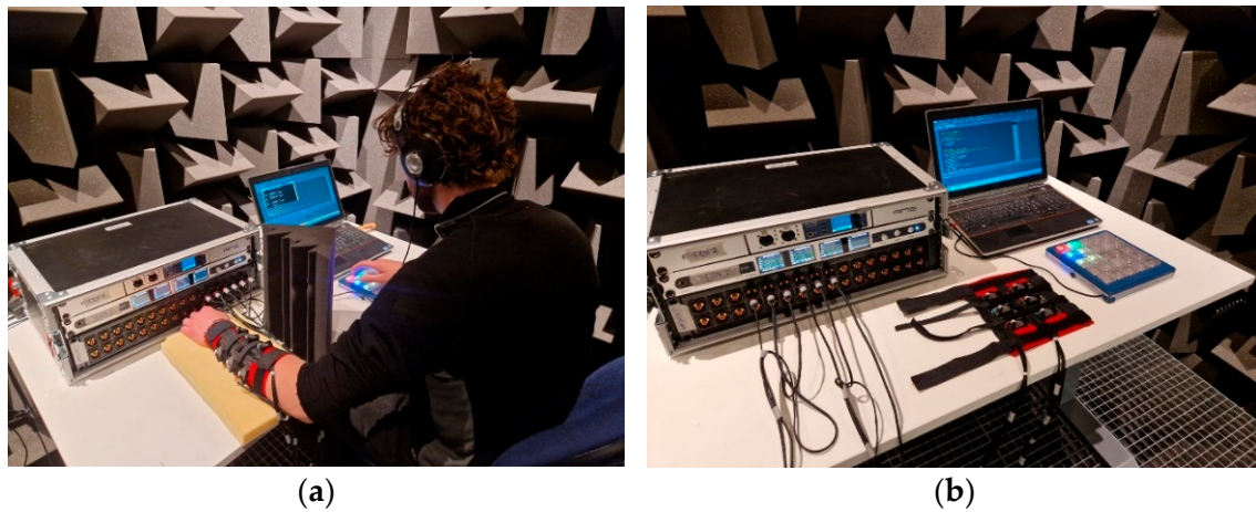
Figure 3. (a) A participant in the anechoic chamber wearing a vibrotactile sleeve, with his hand resting on a cushion. The participants wore headphones playing white noise to block out external auditory cues and responded to the vibrotactile feedback by pressing the correct keys on the keypad. (b) The audio hardware consisted of a digital audio interface (RME MADI face XT), digital-to-analog converters (Ferrofish A32), multi-channel amplifiers, and parallel vibrating voice coil actuators (Lofelt L5), t L5). The MADI face XT receives information from a computer via a USB cable and sends the signal to the Ferrofisch A32 Analog-to-Digital/Digital-to-Analog (AD/DA) converter. Ferrofisch A32 then conveys the signal to the amplifier, which then sends the amplified signal to the actuators.
