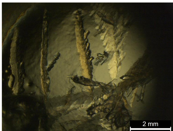
Figure S23. Plate-shaped crystals (with a herringbone pattern) of metronidazole (50 mg/mL) formed in L-phenyl alanine methyl ester based bis-(urea) gel in nitrobenzene at 2.0 wt/v%.
