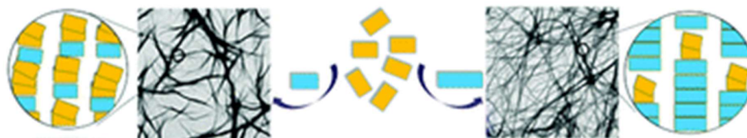
Figure 1.25 Yellow block represents donor moiety, and blue blocks represent acceptor moieties, dense fiber formation with less width when the size of the blue block was large. 171
