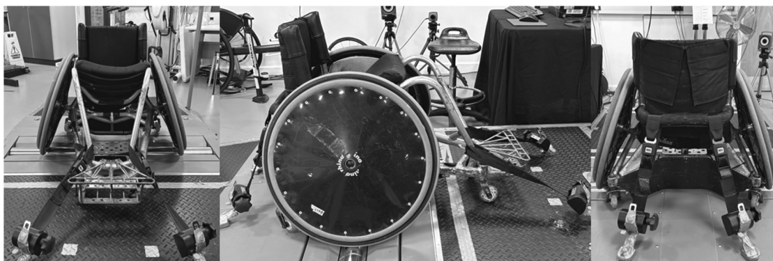
Figure 1. Experimental setup of the dual-roller wheelchair ergometer.
