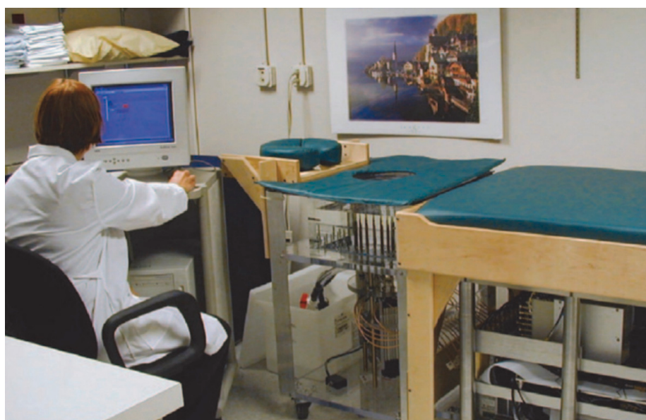
Figure 5. Microwave tomography at Dartmouth College [49]. Image from articles published under an open-access Creative Common CC BY license.
