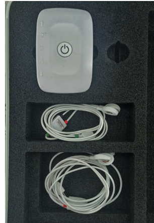
(b) Wireless 4-channel HUB and sensor cables
