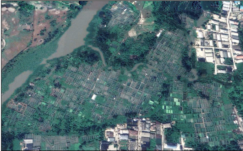
Fig. 1. Google Earth imagery of a fish farm cluster in Nigeria covering about 30 hectares with many small pond units (the smaller ones are about 70 m 2 each). Each farmer may have 1 to 5 ponds in the cluster. Measurements made using Google Earth measuring tool.
