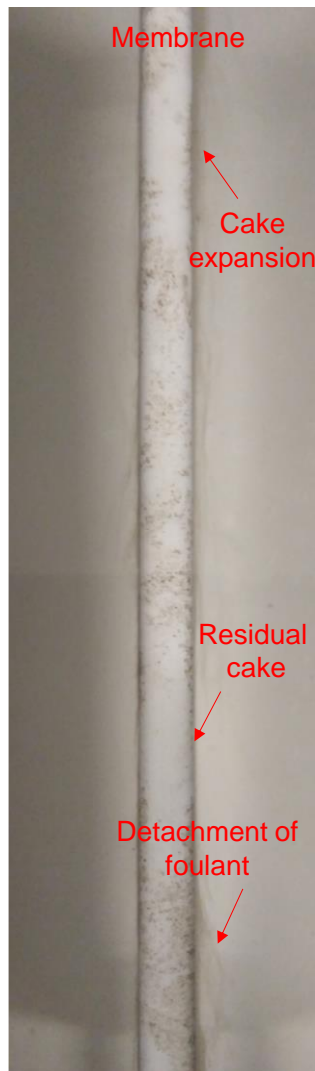
Figure 3.10. Photo of the fouled membrane during ultrasonication in the GDM system (after 3-h filtration).
