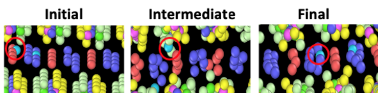
Figure 5.4: Visualization using the OVITO software to outline the vacancy migration when the displaced iodide is within one unit cell of the vacancy. The large blue sphere between two mid-sized red ones indicates the vacancy (pseudo-particle) and under-coordinated Pb atoms, respectively.
