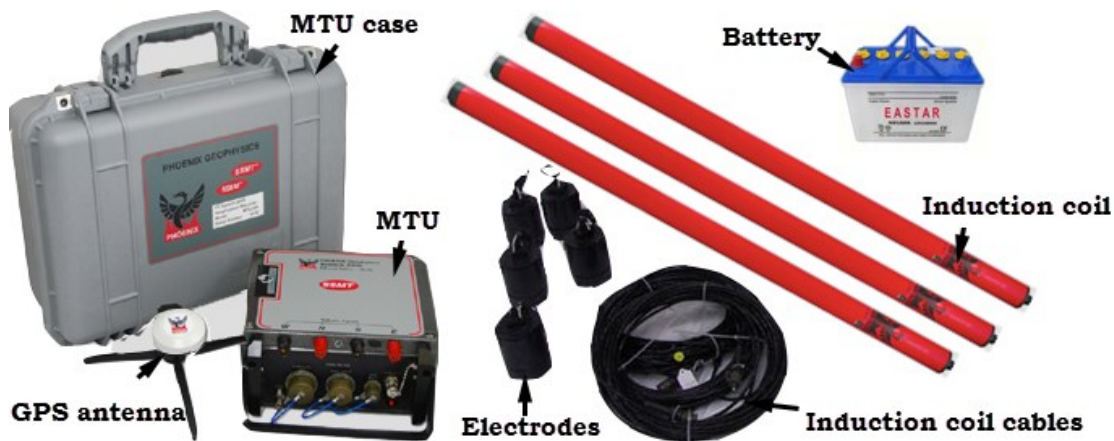
Figure 2.3 Phoenix MTU-5A system (Phoenix, 2018) used for the data acquisition.
