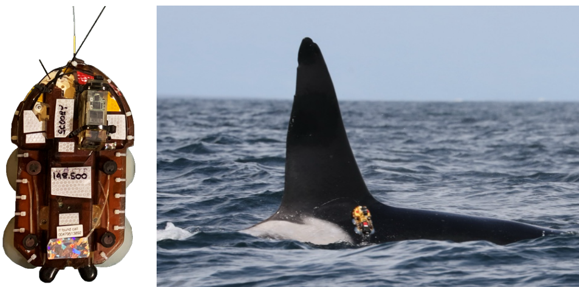
Figure 7: Dtag in the lab and attached to a killer whale (photo: Tatiana Marchon).
