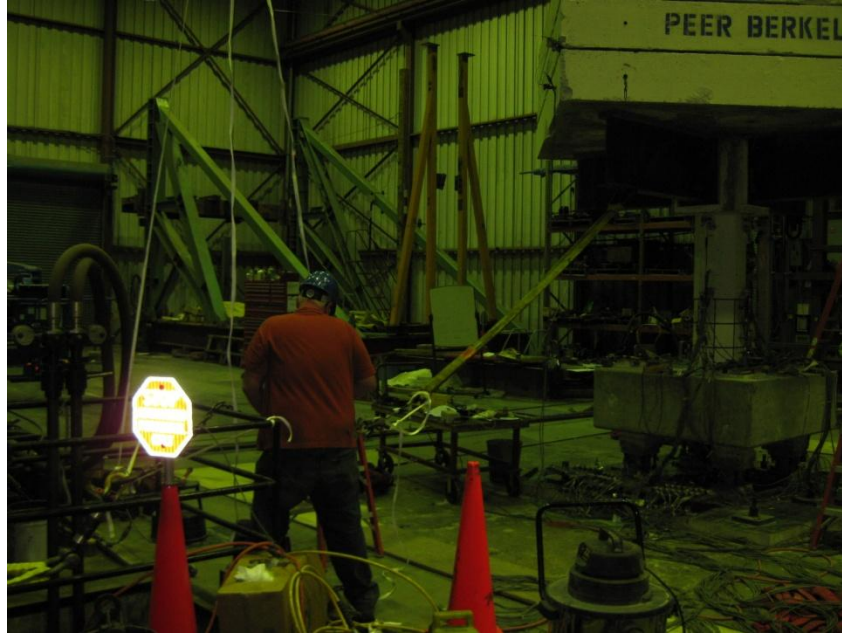
Figure 6-19. Cable being cut in a free-vibration test
