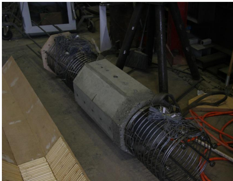
Figure 6-5. Specimen PreT-SF-FIB-SHK before installation in prestressing rig
