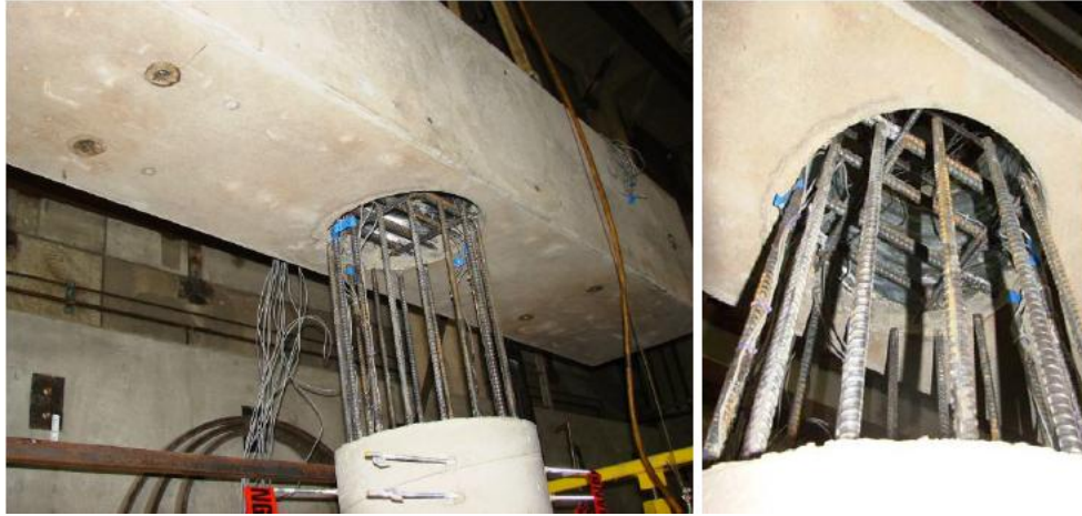
Figure 2-6. Assembly of the “pocket” connection (Matsumoto 2009)
