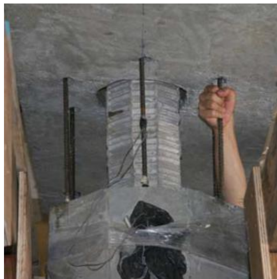
Figure 4-5. PreT-CB-CONC column-to-cap beam connection (Davis et al. 2012)
