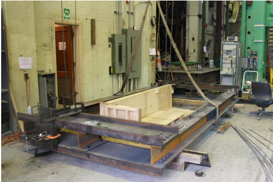
Figure 6-7. Prestressing rig fabricated for Specimen PreT-SF-FIB-SHK
