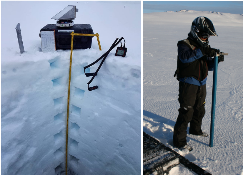
Figure 2.8. Left: A typical snow pit where detailed density and temperature have been collected at a range of depths, allowing for SWE determination. Right: Collection of depth and bulk SWE data using the Federal snow sampler. Photos by Andri Gunnarsson.
