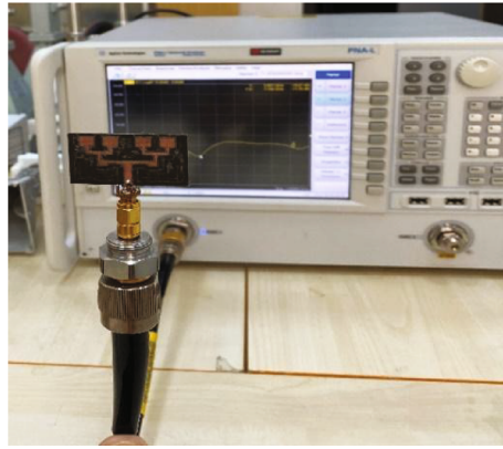
(a) Measurement setup with VNA
