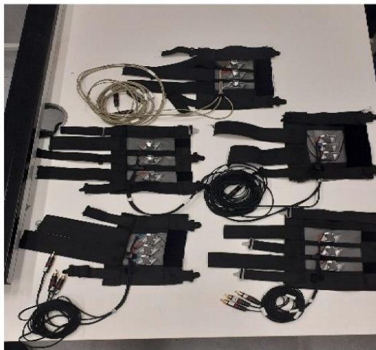
Figure 1. The apparatus used in the study of our research group. Sleeves with different distance between actuators.
