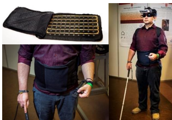
Figure 2. The apparatus used in the SOV device of our research group. Left top photo: The tactile belt prototype version 4 from our Sound of Vision project. Left down photo: closer view on the prototype version 4. Right photo: A person wearing the prototype version 4.
