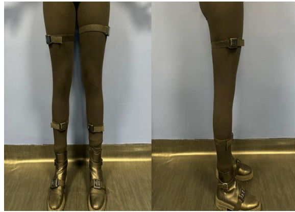
Figure 2. Position of the OPAL wearable sensors on the lower limbs to measure the knee and ankle joint angles.
