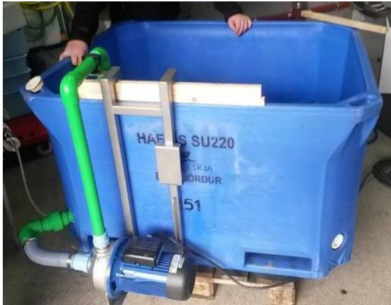
Figure 1: 1000L tub for onboard RSW trial.
