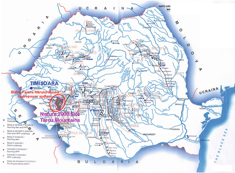
Fig. 18 Hydropower plants in operation (black dots) and under construction (red dots) in Romania. The Bistra - Poiana Mărului - Ruini hydropower system is marked with a red circle [12]
