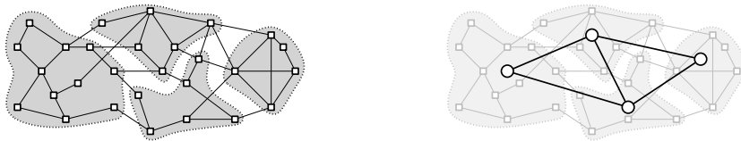
Figure 1. A communication graph G with 4 clusters (left), and the associated cluster graph H (right).
