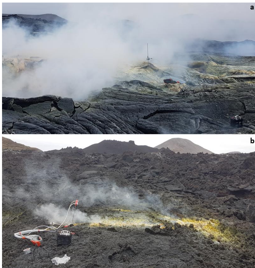
Figure 2.3. Photos of post-eruptive lava gas sampling showing the two set ups used. (a) One filter pack made of both PTFE laminated filters for aerosol collection and base impregnated filters, connected to the 83 L/min Dustbuster® pump. The photo corresponds to the sample GD-2, collected on a lava channel, 1 km SSW of the main 2021 eruptive vent. (b) Two separated filter packs touching each other and connected by tape to collect very similar gas. The laminated filter is connected to the 83 L/min Dustbuster® pump whereas the base impregnated filters are connected to the SKC® 11 L/min pump. The photo corresponds to the sample MD-8, collected on the Meradalir lava field, 100 m N of the main 2022 eruptive vent.
