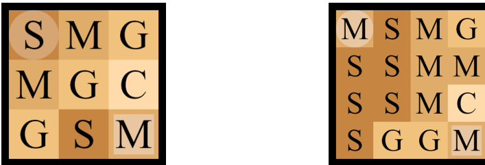
Figure 7.7 – Grid worlds models. (Left) a 3x3 deterministic model; (Right) a 4x4 non-deterministic model.
