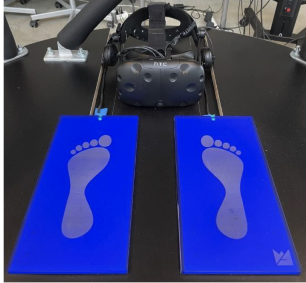
Figure 2.6: Force plates embedded into platform
