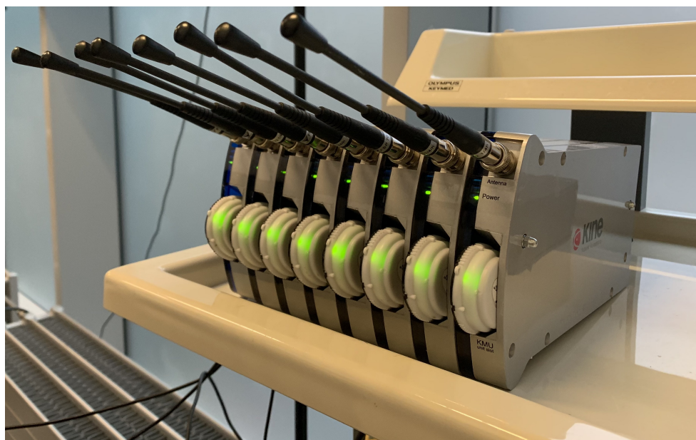
Figure 2.4: Base station for charging wireless EMG sensors
