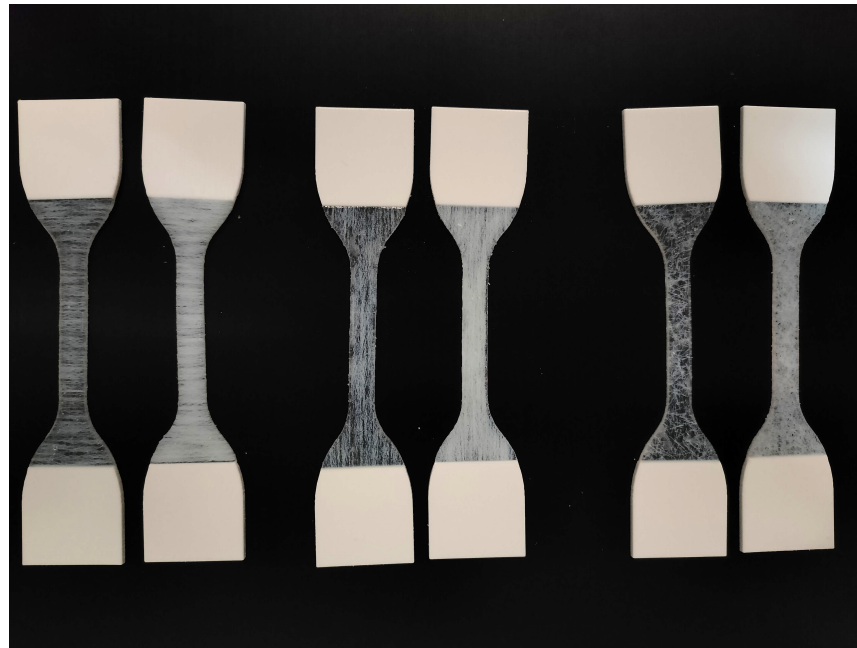
Figure 1. Standardized samples (ASTM D638) with different fiber orientations and concentrations. From left to right, respectively, we have the following: Superficial (1% and 5%), Deep (1% and 5%), and Middle (1% and 5%).
