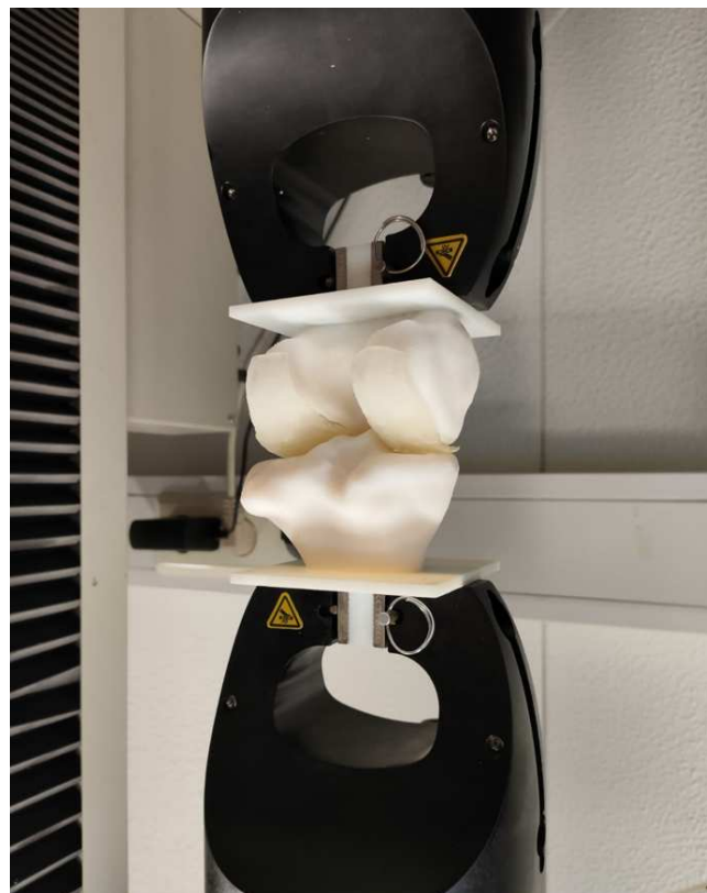
Figure 2. Three-dimensionally printed functional model of the knee joint (femur, tibia and femoral cartilage) during the mechanical evaluation.
