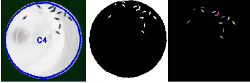
Fig. 3. The image processing steps from left to right—left: vial segmentation; center: threshold image; right: resulting clusters.
