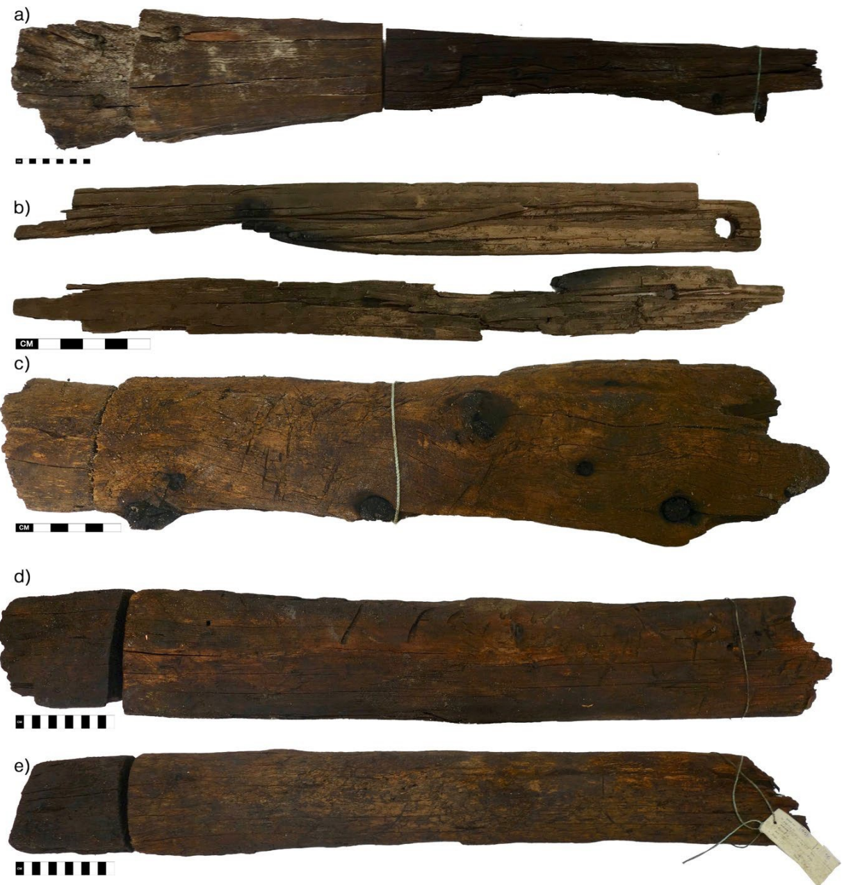
Figure 64. Examples of construction timber from GUS and Tatsip Ataa. a) A construction timber from GUS (X38) – spruce sp. b) A construction timber from Tatsip Ataa (X1489) – spruce sp. c) A post from GUS (X273) – spruce sp. d) and e) A post with ringholes from shipworms ( Teredinida ) from GUS (X255) – larix sp.
