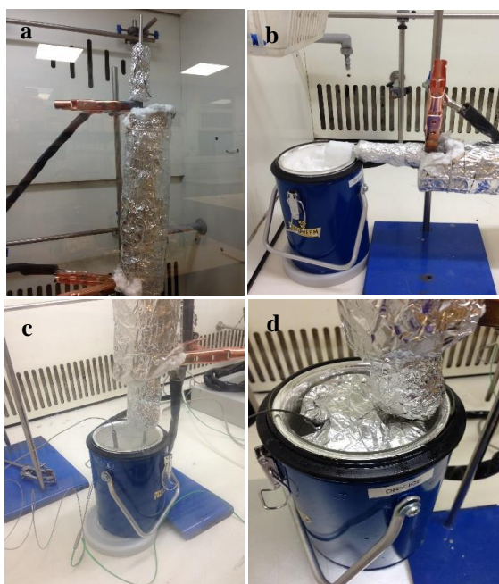
Figure 7: Stainless steel tar tube without cooling bath (7.a), tar tube had placed on top of the cooling bath containing dry ice (7.b), U-shaped tar tube in the cooling bath (7.c), fully insulated cooling bath with U-shaped tar tube (7.d).
