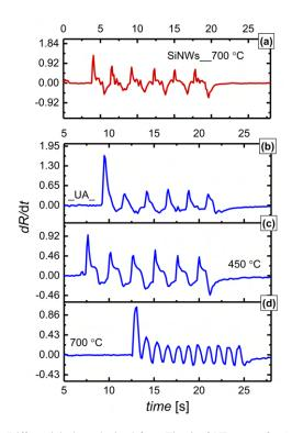
Fig. 4. Differential plots obtained from Fig. 3 of NB states for (a) SiNWs annealed at 700C°C (b) UA-Ge:SiNWs and annealed Ge:SiNWs at (c) 450  $^\circ C$  and (d) 700°C, prospectively.
