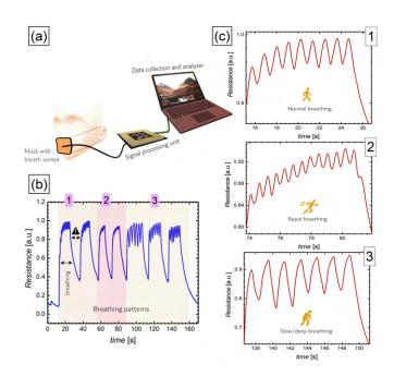
Fig. 5. (a) Schematic of the respiratory setup utilized. (b) The breathing response in real time recorded using annealed ( $700^{\circ}$ C) Ge:SiNWs. (c) The data marked as 1, 2 and 3 expanded.
