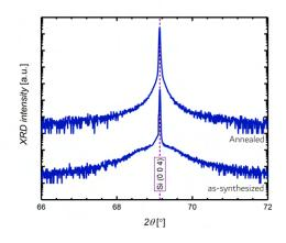
Fig. 2. XRD diffractorgram along Si (004) atomic plane obtained over SiNWs based structures both in un-annealed (lower plot) and annealed (upper plot) state.
