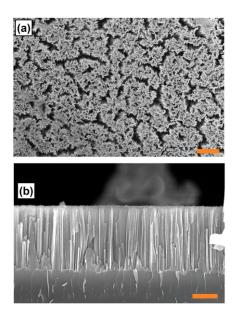
Fig. 1. (a) Top-view and (b) cross-sectional SEM micrograph of SiNWs obtained by MACE. The scale bar provided is  $2\mu m$ .
