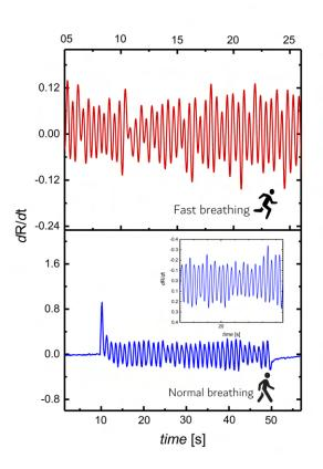
Fig. 6. Differential plot for Ge:SiNWs structure annealed at  $700^{\circ}$ C, 5 min, under RB (upper plot) and NB (lower plot) modes for an increased number of cycles. The sensor was tested again under similar condition for repeatability the results from which are shown in an inset for NB mode.
