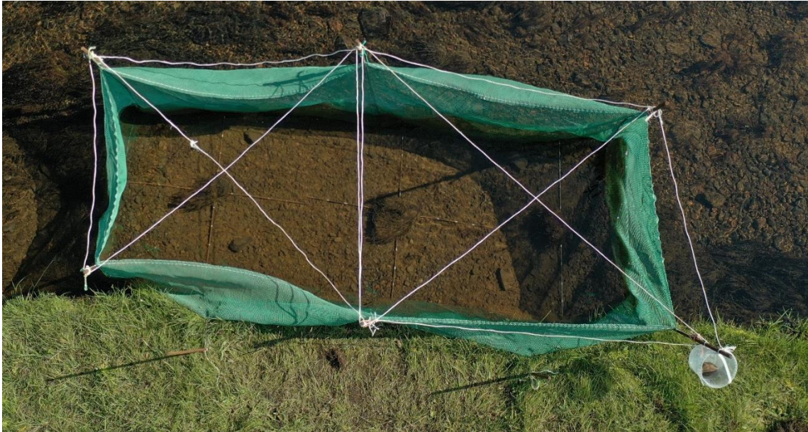
Figure 9. Stream enclosures with metal bars on the bottom indicating grids with 10cm markers (grey tape), three cobbles with moss functioning as shelters and white strings to prevent predation. Photograph credit: Kári Heiðar
