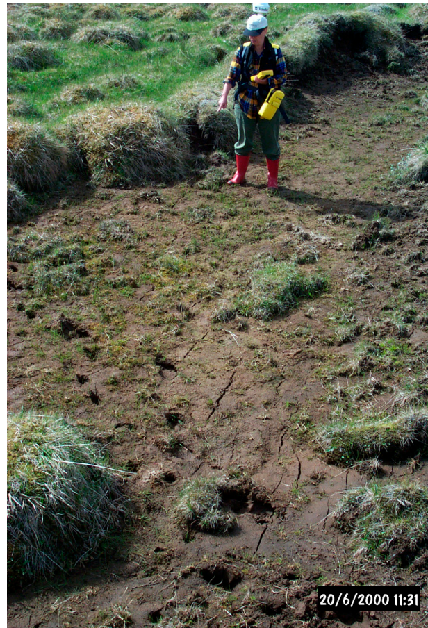
Figure 2. Photograph of fine-scale, en echelon fracture pattern in the source area of the SISZ earthquake of June 17, 2000. – Skástígur sprungur í moldarflagi á upptakamisgengi jarðskjálftans 17. júní 2000.
