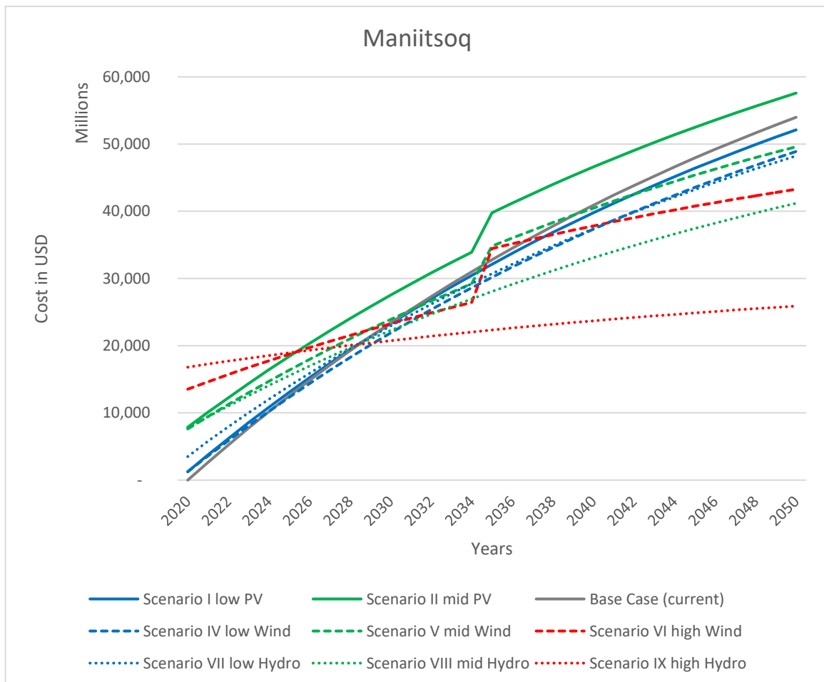
Figure 4. Scenario analysis of possible power generation for Maniitsoq shows the accumulated net present value of cost for power generation with a diesel price of 0.85 $/l; capacity factor of 28%; and fuel consumption of 0.25 l/kWh. The other input data are explained in Table 1, and the scenarios are presented in Table 2. The current setup is close to the base case; Maniitsoq has 0.1% renewables in the mix.
