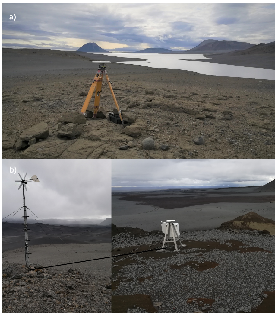
Figure 1.1. (a) Campaign and (b) continuous GNSS equipment set up in the field. For campaign GNSS (a), an antenna is installed on a tripod, above a benchmark, typically measured yearly or every few years. A receiver is connected to the antenna (inside the black box) to shelter it from bad weather. Continuous GNSS in Iceland (b) typically has an antenna installed on a quadropod. The receiver is in a box, connected to electricity. In Iceland, the continuous GNSS stations normally obtain electricity from a wind turbine and a solar panel.
