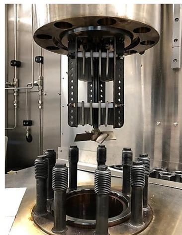
(b): The autoclave with the lid opened shows 8 mounted test samples.
