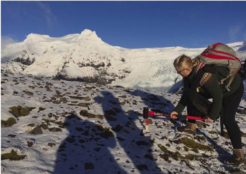
Figure 4: A local member of the scientific monitoring mission to the slope instability hammers a metal stake into the ground. The exact GPS position of the stake is one of several methods being used to measure changes in the width and position of the slope (Photo: Stephanie Matti, 2018).
