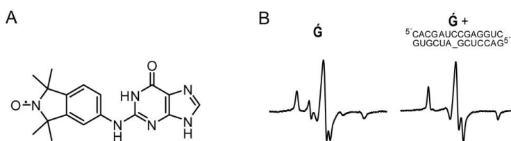
Figure 2.5. (A) Structure of \dot{G} (B) CW EPR data of \dot{G} (left) and \dot{G} bound to a RNA duplex containing an abasic site at -20^{\circ}\text{C} (right).
