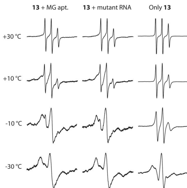
Figure 3.7. EPR data for the isoindoline-derived MG 13 bound to the aptamer (left column), mutant RNA (middle column) and without any RNA (right column). EPR spectra were recorded as a function of temperature. All data were recorded in 10 mM phosphate, 100 mM NaCl, 0.1 mM Na 2 EDTA, pH 7.0.
