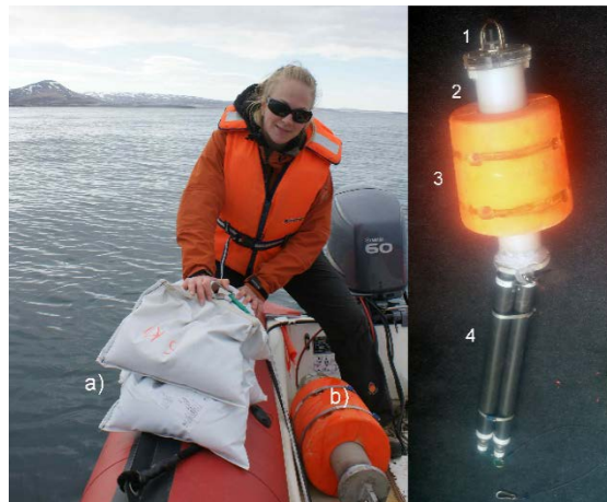
Figure 4 An EAR unit ready for deployment in Skjálfandi Bay by Edda E. Magnúsdóttir, NE-Iceland. Left: a) sandbag weights (~45 kg) were connected to the EAR unit by a 1 m long and 3mm wide rust-free wire, b) the EAR unit. Right: 1) The hydrophone, 2) an aluminium housing, 3) a syntactic foam float and 4) two acoustic release units. Left © Yann Kolbeinsson, right © Edda Elísabet Magnúsdóttir
