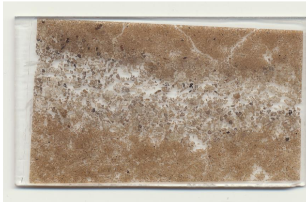
Fig. C4: Thin section of tephra in situ, soil above and below is the brown finer grained material while in the center the tephra layer is preserved. Up direction on the thin section corresponds to the up direction for the tephra layer as seen in soils.
