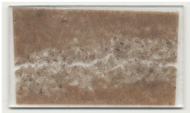
Fig. C5: Another thin sectioned tephra layer, this illustrates how the tephra layer is a weak point in the structure and confinement is needed during preparation.
