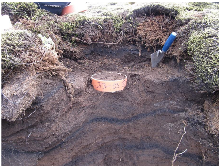
Fig. C1: Sampling method of tephra by tube, the soil above and below the tephra layer preserves it in situ.
