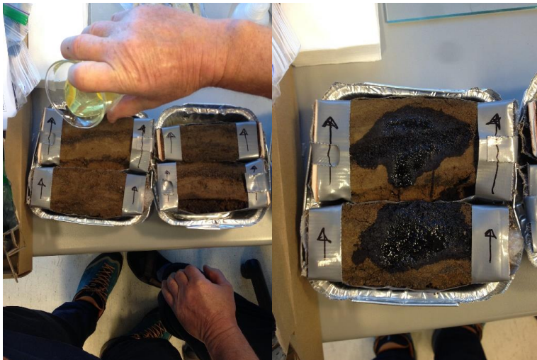
Fig. C3: Preparation for thin-section. Epoxy was poured over soil and tephra. When epoxy had set loose material (i.e., soil and tephra) was removed and thin-section prepared. Orientation of the tephra layer was always documented.
