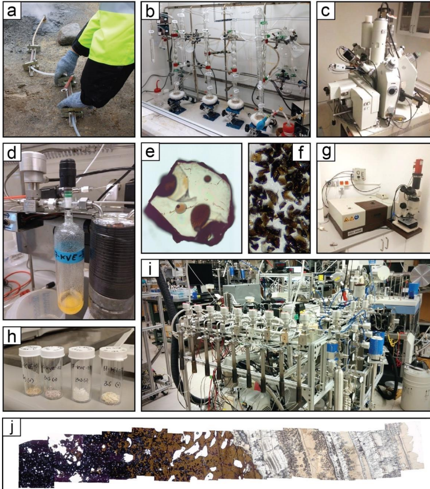
Figure 1.3 Methods (a) Sampling fumarole gas into duplicate copper tubes for noble gas analysis. Víti, Askja. (b) Sulfur extraction setup at IES. (c) Electron probe microanalyzer at the Institute of Earth Sciences. (d) A fumarole sample in a two-port “Giggenbach” bottle hooked into the inlet system of a gas chromatograph at IES. (e) View of an olivine crystal from Kverkfjöll with four visible melt inclusions. The exposed melt inclusion has a vapor or shrinkage bubble. (f) Glass shards from subglacial pillow basalt rims, crushed, cleaned and sieved preparation for \delta D analysis. (g) Fourier-transform infrared spectrometer used for analysis of H_2O-CO_2 contents in glass and melt inclusions, IES. (h) Fumarole gas H_2S precipitated has ZnS in preparation for S extractions. (i) The custom-built fluorination and purification inlet system for multiple sulfur isotope analysis at MIT, USA (j) A thin section image of a subglacial pillow basalt with crystalline interior (dark), glassy rim (bottle brown), and travertine layers (white-beige) precipitated from the Hveragil thermal river, Kverkfjöll.
