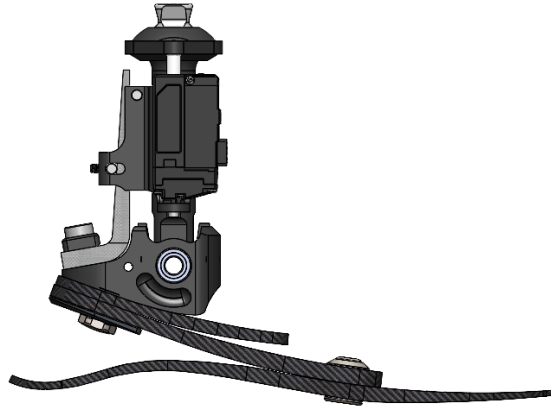
Figure 5-8. Schematic of future design evolution of VSA prosthetic foot.
