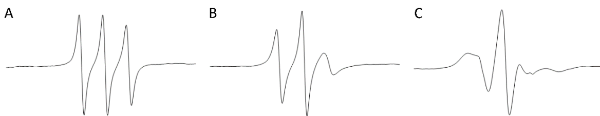
Figure 5.6. CW-EPR spectra of free nitroxide \dot{C} (A), spin labeled DNA oligonucleotide XIV (B) and spin labeled DNA duplex J (C). EPR spectra were recorded at 22 °C in a phosphate buffer (2 nmol of sample; 10 mM phosphate, 100 mM NaCl, 0.1 mM Na 2 EDTA, pH 7.0).
