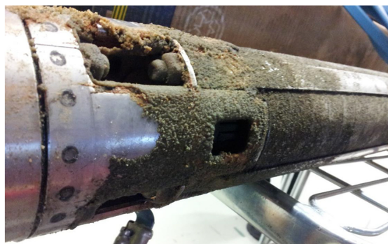
Fig. 4. Photograph illustrating the presence of precipitates on the water sampling pump recovered from monitoring well HN-04 on the 13th of August 2013. The diameter of the pump is 101 mm. (For interpretation of the references to colour in this figure legend, the reader is referred to the web version of this article).
