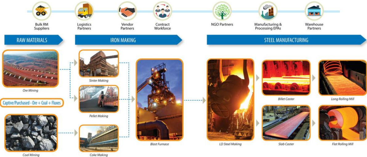
Figure 2.1.4.14 - Crude steel production Value Chain, adapted from (Tata Steel, 2014).
