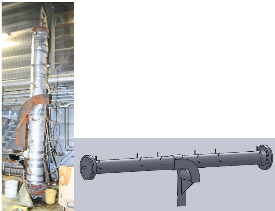
Figure 3.16: A photo showing the experimental setup and a 3D drawing showing the pipe on the steel bracket.
