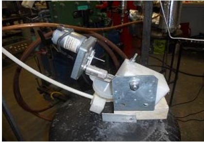
FIGURE A.2: Particle feeding (left) and ejector assembly (right)
