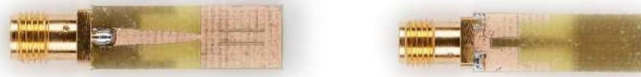
FIGURE 2 Photographs of the fabricated antenna prototype. A, Top layer, and B, bottom layer. [Color figure can be viewed at wileyonlinelibrary.com]
