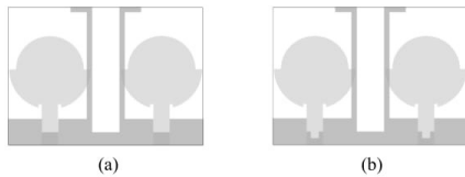
FIGURE 3. Evolution progression of the considered UWB-MIMO antenna. The ground plane is shown using the dark gray shade. (a) Antenna II, (b) Antenna III.
